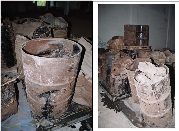
Tarry wastes leaking from old and damaged barrels.
